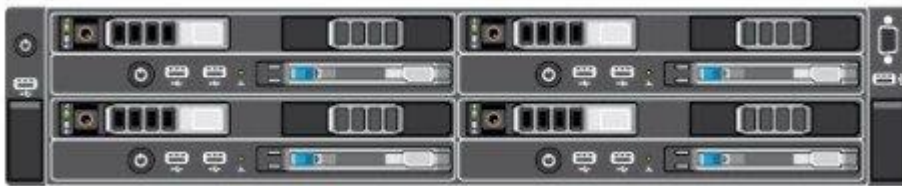
Figure 5. Front View with Server Modules
