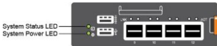
Figure 3. System LEDs on Front Panel
